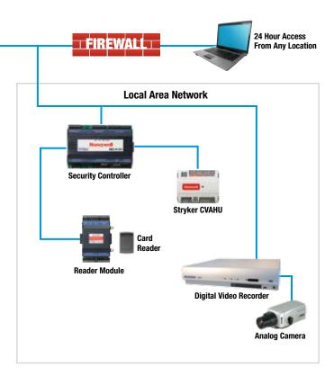
**BUILDING 3 (Compact Security Solution):** The Compact Security Solution provides security and HVAC control — ideal for smaller buildings or when adding another controller doesn't make sense.
