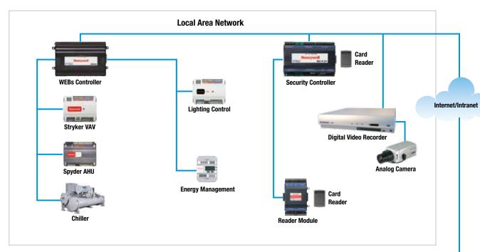
**BUILDING 1:** Includes HVAC control, DVR, access control and energy management for a comfortable, secure and energy sensitive building.
